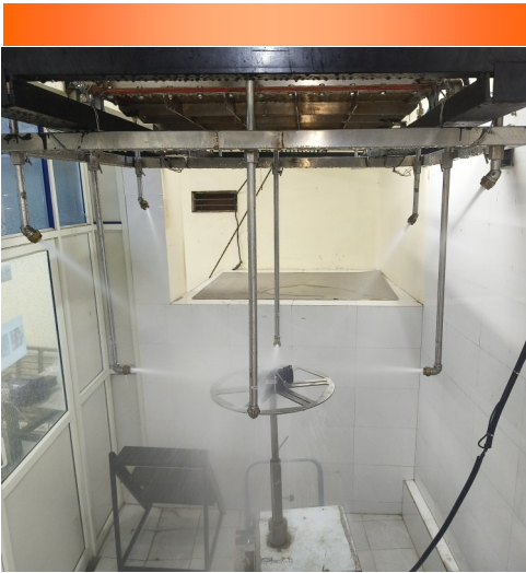
Real-time image of a water ingress test in progress at Envitest Lab.
