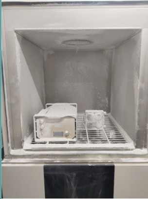
At Envitest Lab, the IP dust test checks how well a device keeps out dust particles, ensuring it meets protection standards.
