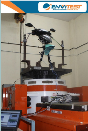
Testing for durability and reliability of an automotive component at Envitest Lab.
