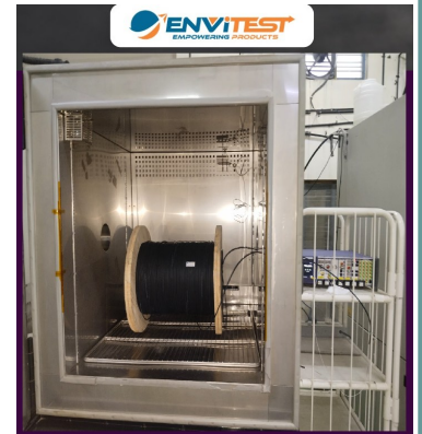
Measurement of Insertion Loss (IL) and Return Loss (RL) in fiber optic cables, using advanced tools to ensure accurate testing for quality control, network maintenance, and research.
