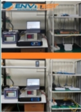
Test setup in action at Envitest Lab, performing TEC ECR testing to evaluate the energy consumption and efficiency of telecom equipment
