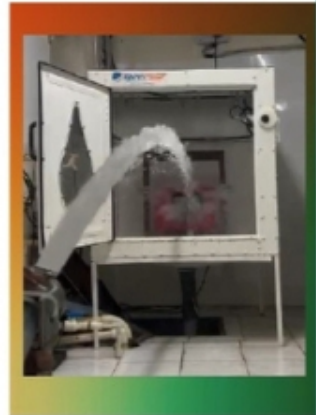
Hose Down Test is running live, splashing water at a rate of 240 liters per minute from a distance of 3 meters.
