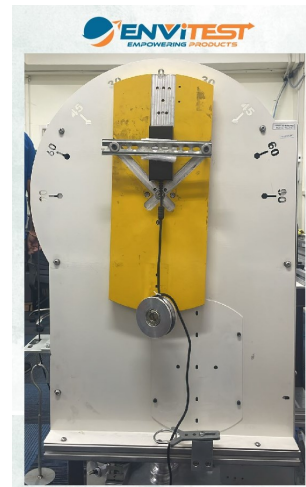
The repeated bending test setup at Envitest
