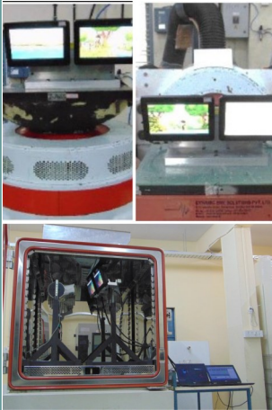
Evaluating the performance of electronic components under extreme temperatures,
