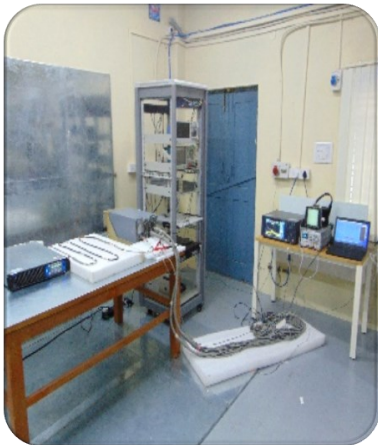
"Testing setup for full capability MIL STD 704 on an engineering product at Envitest Lab Live!"
