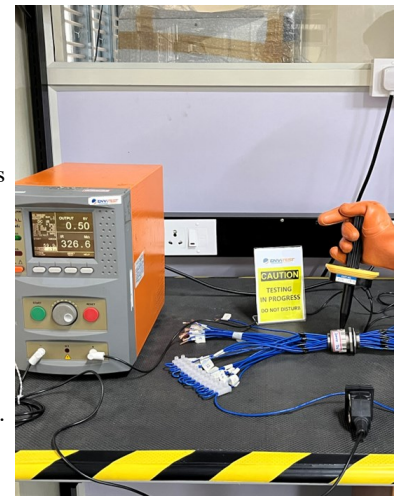
Insulation Resistance test verification in real time at Envitest lab
