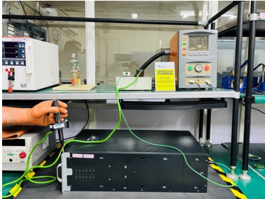
“Laboratory test setup for measurement of Ground Bond test at Envitest Electrical lab—Live!”
